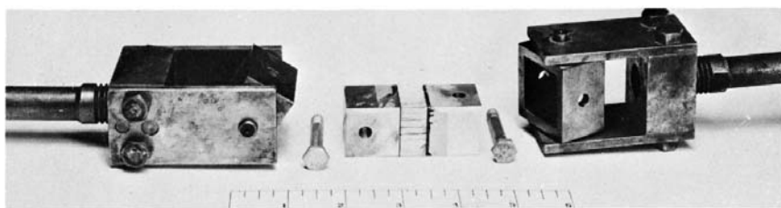
FIG. 4 Grip Assembly for Type B Specimen
