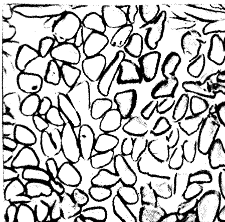
FIG. 5(b) RAW SILK — CROSS-SECTIONAL VIEW ( \times 500 )
