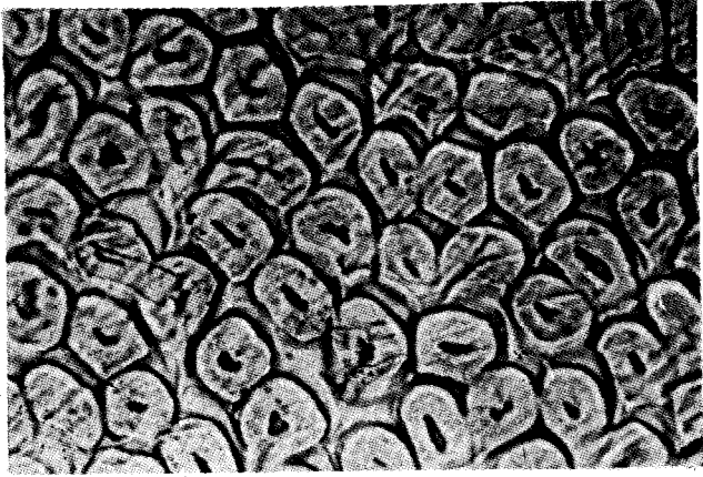
FIG. 11(d) POLYESTER, HOLLOW — CROSS- SECTIONAL VIEW ( × 500 )
